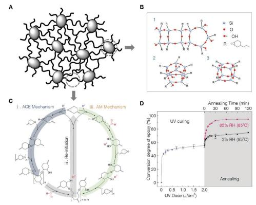
**Figure 1.** Design concept of the ESMH. A) Schematic illustration of the ESMH consisting of nanosized siloxane molecules densely crosslinked by cycloaliphatic epoxy chains. B) Representative molecular structure of the CEOS (1: ladder-like structure, 2: partial cage, 3: cage). C) CROP of cycloaliphatic epoxides by ACE and AM mechanisms with H<sub>2</sub>O molecules as the CTA. D) Epoxy conversion of the CEOS (mean value  $\pm$  SD, N = 10) upon UV irradiation followed by annealing processes.
